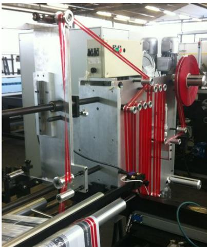
Nastro sicurezza e liner accoppiati con colla / security tape and release liner laminated with hotmelt
